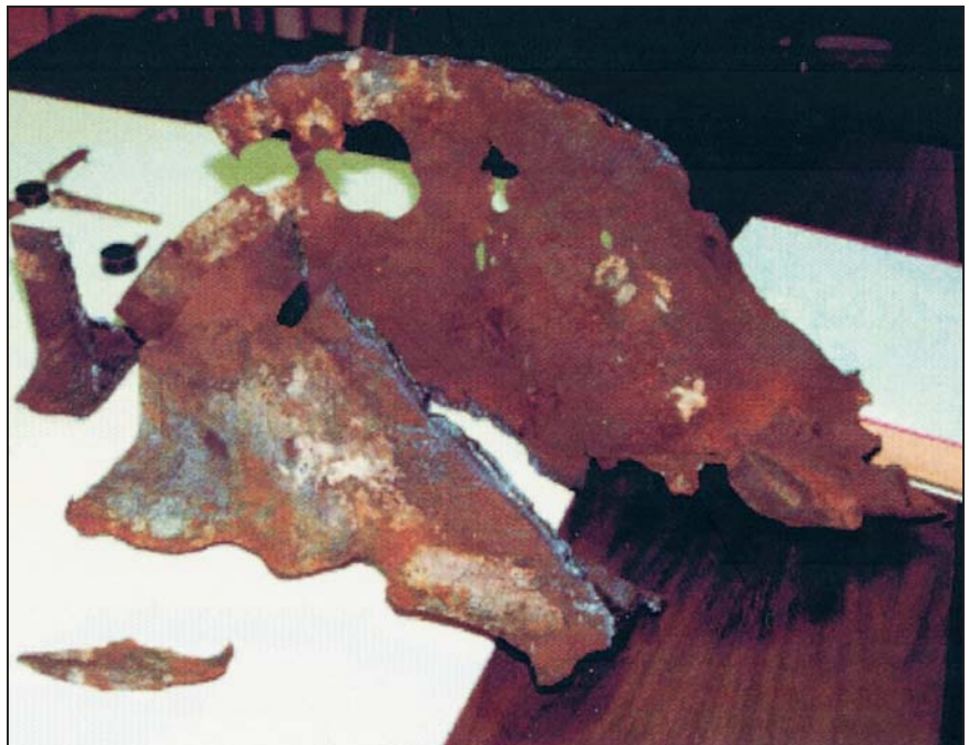
Figure C-1 Eroded A36 wide-flange beam.
