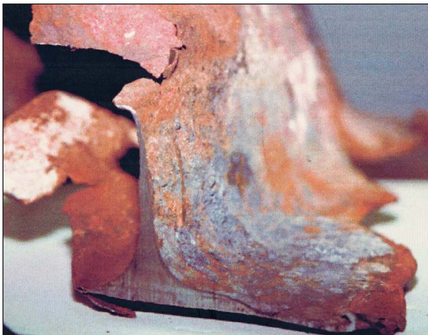
Figure C-2 Closeup view of eroded wide-flange beam section.
