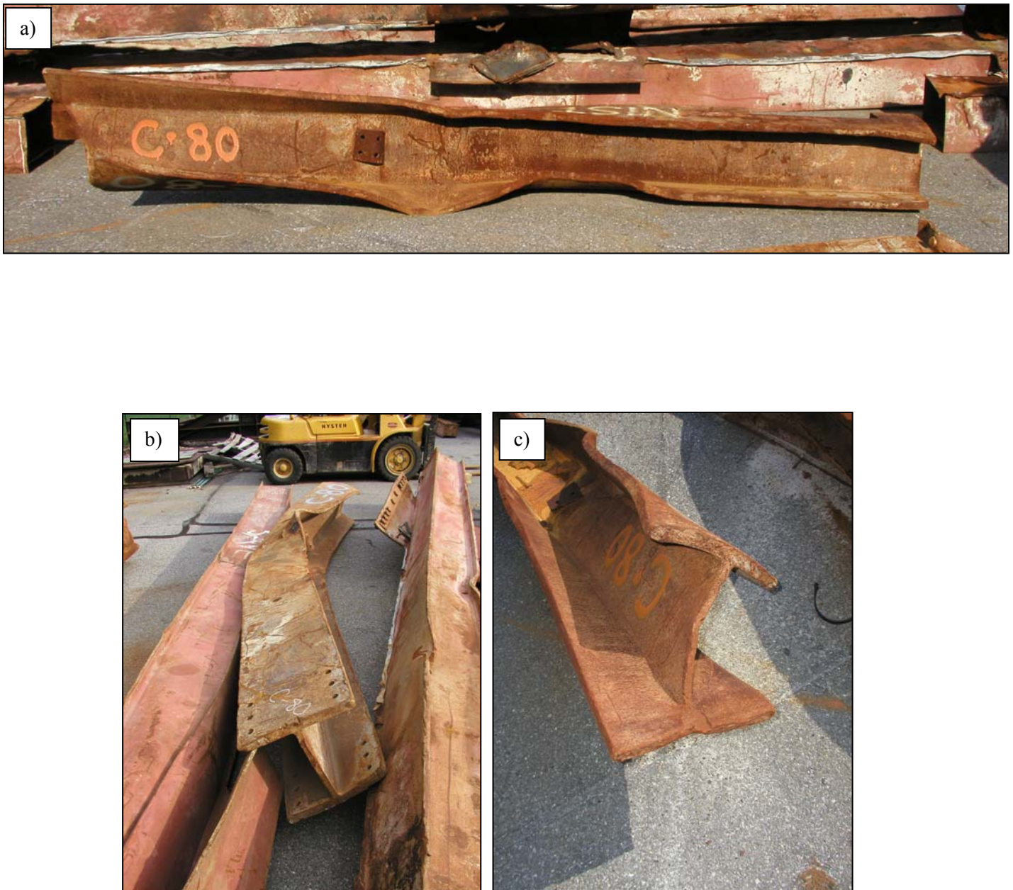
Figure 6–30. Core column C-80 (603A: 92-95). a) Overall view of recovered column, b) view of connection in the 92nd floor region, failure as a result of bolt fracture, and c) torn end of column near the 94th floor region.
