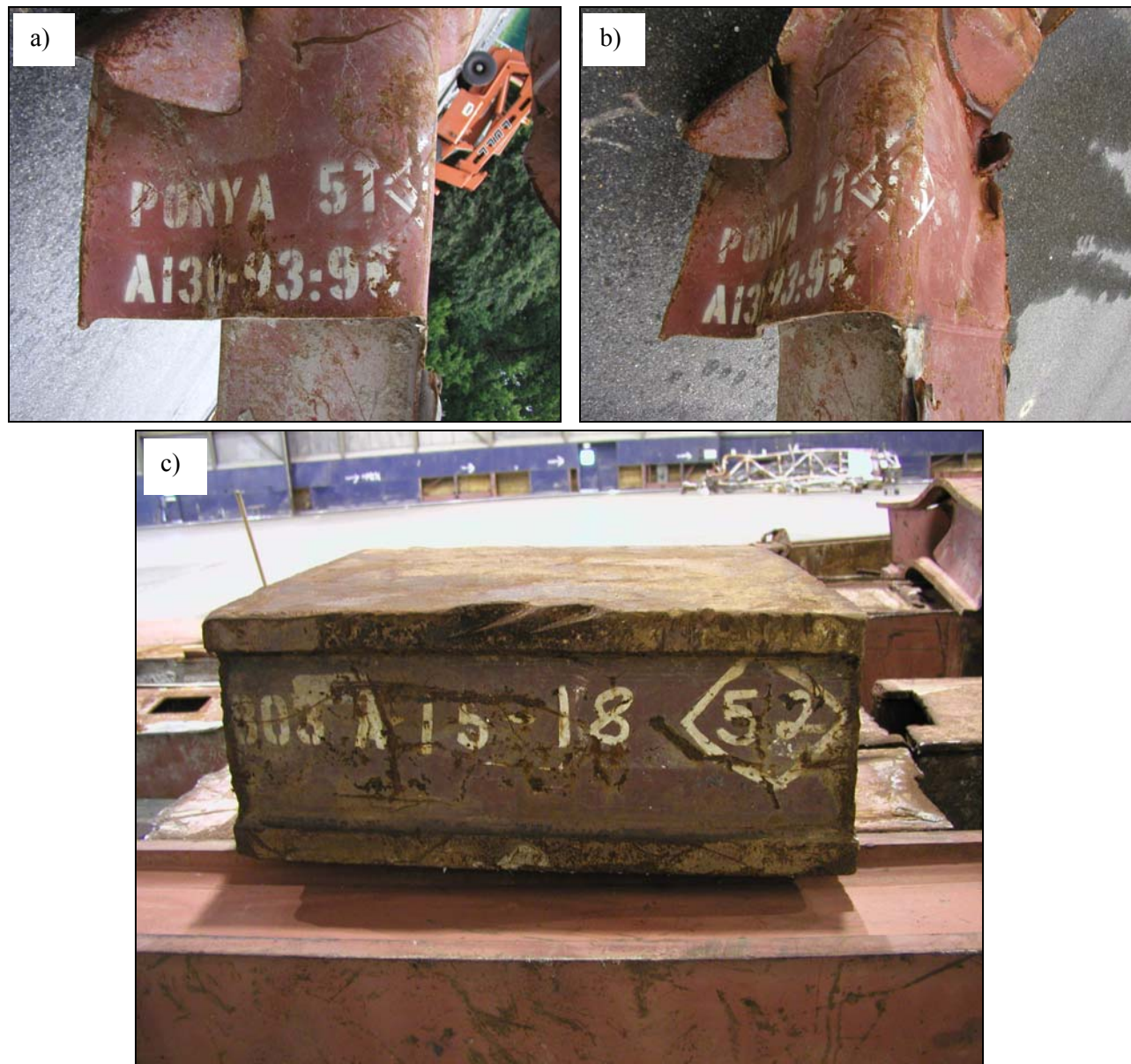
Figure 5–3. a) and b) Characteristic stenciling found on the lower portions of the exterior column panels for sample M-27. Markings indicate this piece was in WTC 1, column number 130, spanning floors 93 to 96. Also seen are two other indicators, “5T” and “<63>,” indicating the estimated piece weight in tons and erector’s derrick division number, respectively. c) Characteristic stenciling found on core column for sample B-6152-1. Markings indicate this piece was in WTC 1, column number 803, spanning floors 15 to 18 with a derrick division number of <52>.
