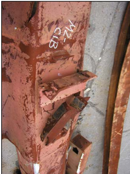
Figure 6–27. Floor truss connectors for panel M-2 (A130: 96-99).
