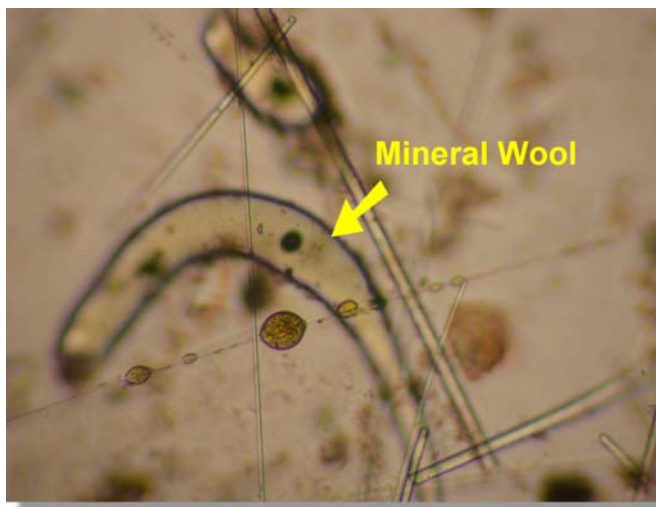
Figure 14. Optical microscopy image of mineral wool fragment.
